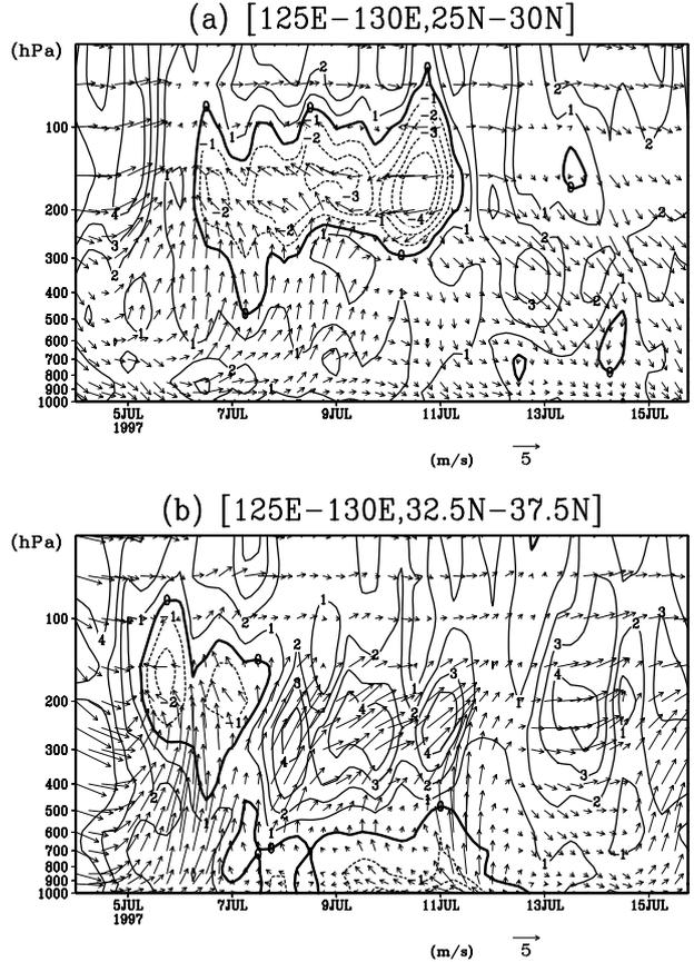
Figure 5: Time-height cross sections of the ageostrophic meridional circulation ( $v_a, w$ ) averaged in the areas of (a) the south side (125–130°E, 25–30°N) and (b) the north side (125–130°E, 32.5–37.5°N) of the Baiu front.
