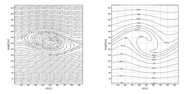
Figure 9.4. Stream function of (u - w) at 240 seconds Figure 9.5. Potential temperature [K] at 240 seconds from the initial.
