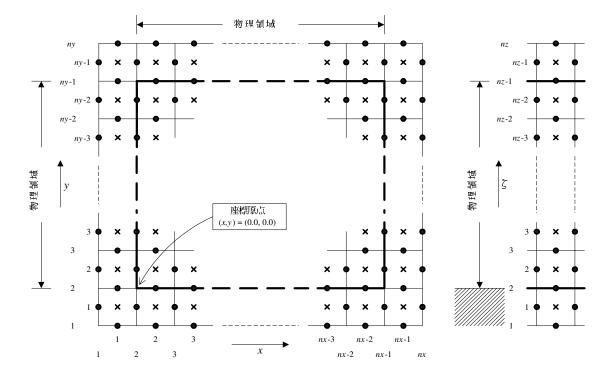
Figure 9.2. Setting of variables in the calculation domain. The closed circles are points of vector variables and the crosses are of scalar variables.
